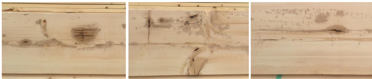
FIGURE 7 – AN EXAMPLE OF “DIESEL ROT” IN NEWLY CUT SPRUCE LUMBER.
